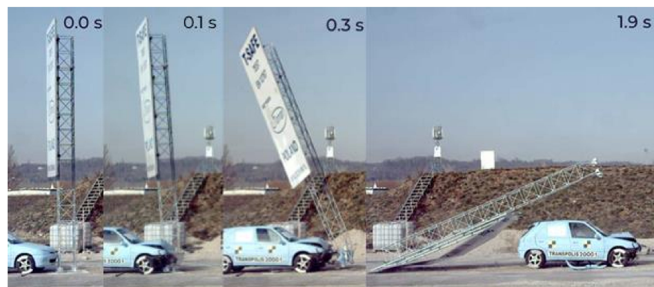
Figure 11. The result of a crash test with T03 mast at 35 km/h velocities.
