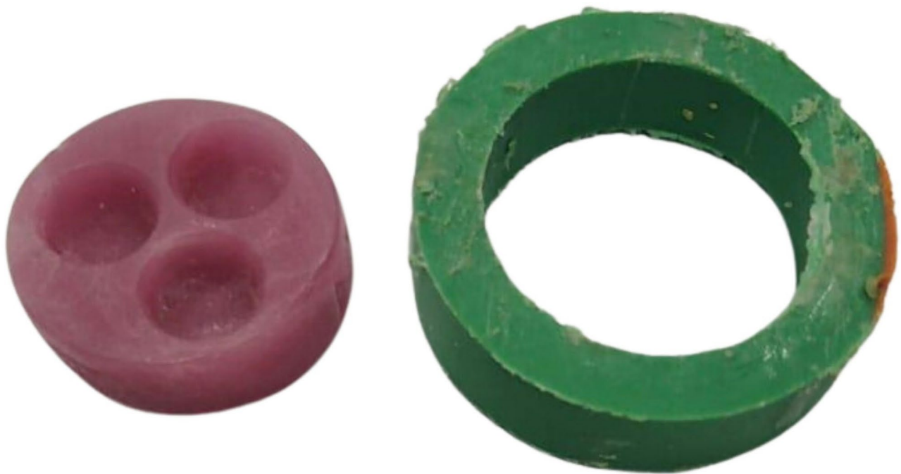
Fig. 1 The mold used to prepare the specimens for the SBS experiment
