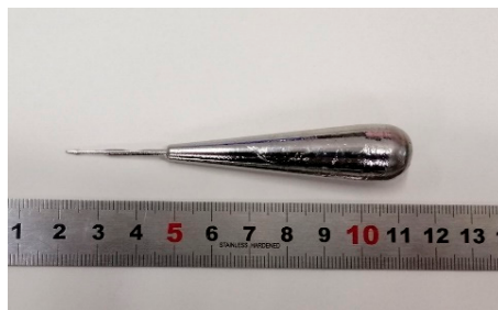
Figure 1. An as-cast conical sample for determining the critical diameter of different alloy compositions.
