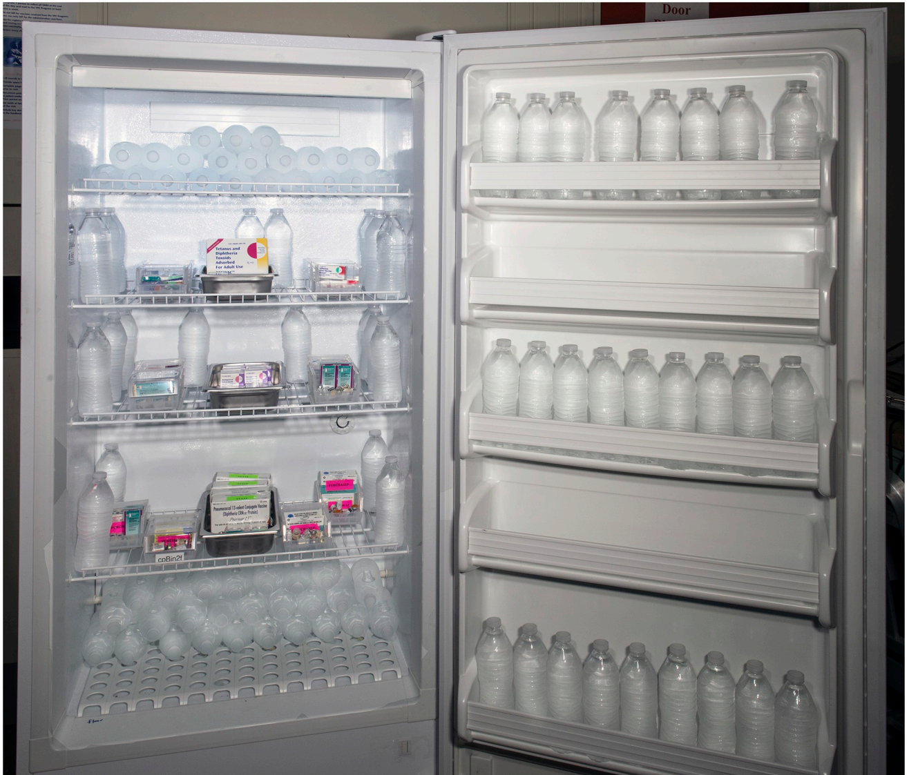
Fig 3. Standalone refrigerator filled with a 10% thermal ballast load comprised of 500 mL (16.9 oz) plastic drinking water bottles. Water bottles were concentrated in door, top shelf, and floor level of the unit, with a small number of bottles placed along the side walls of the unit. The relative distribution of thermal ballast (water bottles), detailed in the text, was kept fixed throughout the study. Plastic and metal bins placed in the center of the unit were used to contain a mix of boxed and unboxed vaccine vials.
