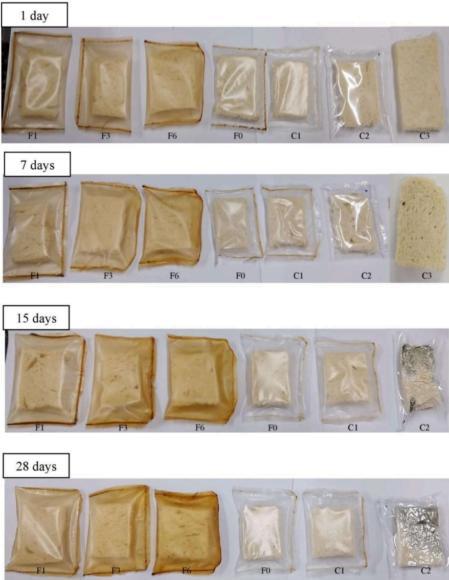
Figure 3. Bread packed: front area. Formulations: F0 (without CC-0.5% CA), F1 (1% CC-0.25% CA), F3 (3% CC-0.5% CA), F6 (6% CC-1% CA), C1 (without CC and CA), C2 (low-density polyethylene), and C3 (unpacked breads, removed after 7 days of storage).
