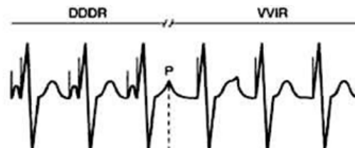
Figure 1. Schematic illustration of EMI-induced conversion to VVI pacing from DDDR pacing mode after electromagnetic interference.
