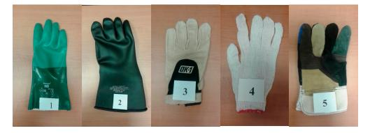
**Figure 2.** Industrial gloves used in the study. Chemical protection glove (**1**); Rubber insulating glove for electrical shock (**2**); Anti-vibration impact glove (**3**); Cotton yarn knitted glove (**4**); RY-WG002 working glove (**5**).
