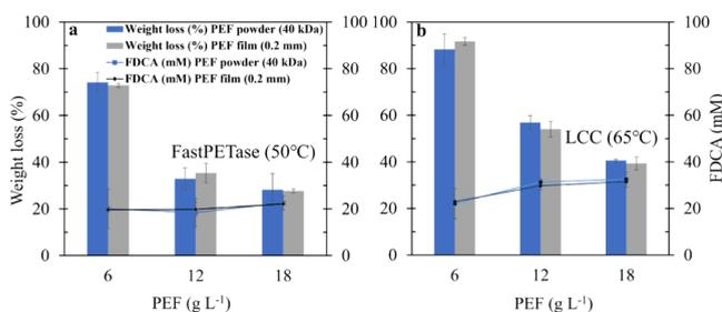
**Figure 3.** Depolymerization (weight loss and FDCA release) profile of PEF powder (40 kDa) and amorphous PEF film (0.2 mm) of (a) FastPETase (20 nM g<sup>-1</sup> PEF) and (b) LCC (80 nM g<sup>-1</sup> PEF) at different substrate concentrations for 72 h. The reaction was performed in 50 mM KH<sub>2</sub>PO<sub>4</sub>-NaOH buffer (pH 9.0).
