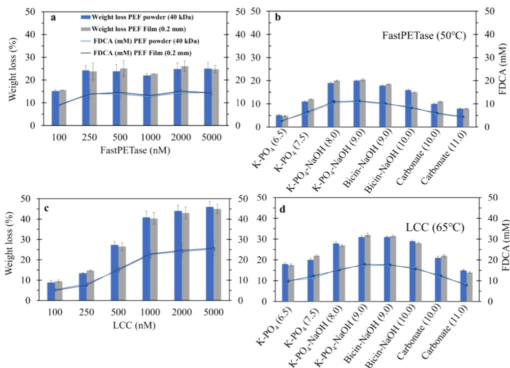
**Figure 1.** Depolymerization (weight loss and FDCA release) profile of  $13 \text{ g L}^{-1}$  of PEF powder (40 kDa) and amorphous PEF film (0.2 mm) using (a) FastPETase at  $50^\circ\text{C}$  and (c) LCC ( $65^\circ\text{C}$ ) using different concentrations (100, 250, 500, 1000, 2000, and 5000 nM). (b) FastPETase ( $50^\circ\text{C}$ ) and (d) LCC ( $65^\circ\text{C}$ ) in different buffers and pH.
