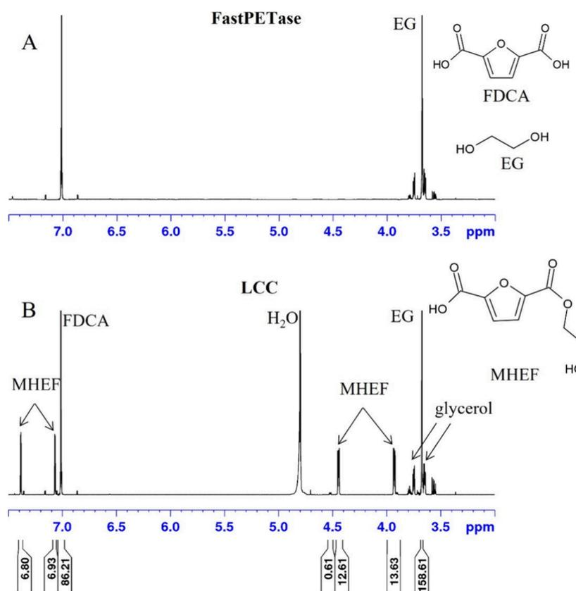
**Figure 6.**  $^1\text{H}$  NMR spectra of supernatant after treatment of PEF with (A) FastPETase and (B) LCC. While the only hydrolysis product detected after FastPETase degradation is FDCA, LCC produces  $\sim 14\%$  MHEF and  $\sim 86\%$  FDCA under the conditions used. Other minor reaction products exist and could be detected by LC-MS (see Figure 5 and Figure S3).
