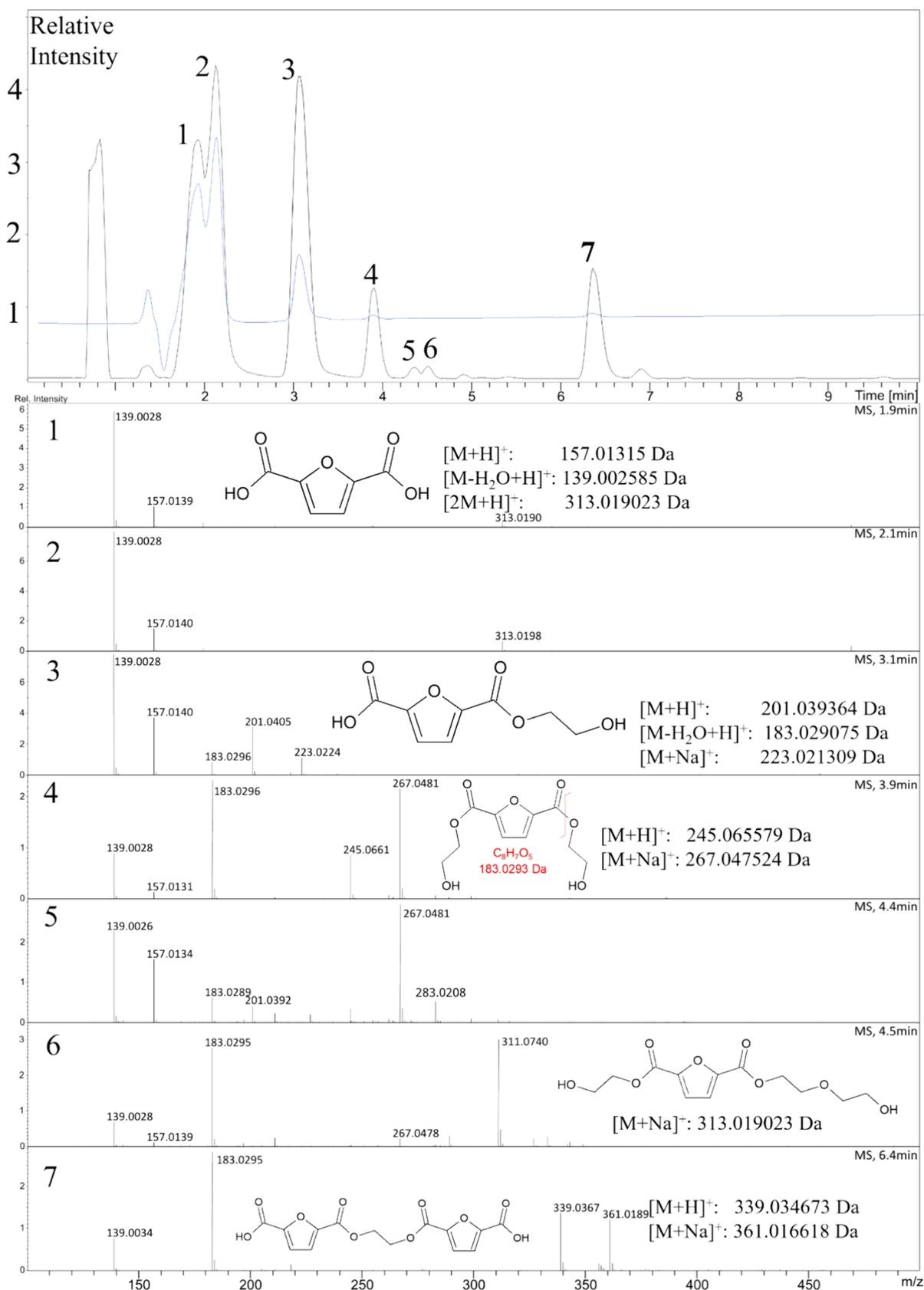
**Figure 5.** LC-MS analysis of LCC-catalyzed PEF depolymerization products after 24 h. Blue line: UV-chromatogram at 243 nm; black: base peak chromatogram (MS, positive mode). The mass spectra at the seven indicated peaks with possible structures to fit the observed masses and possible structures are shown. FDCA is eluting in two separate peaks; the reason for this is unknown.
