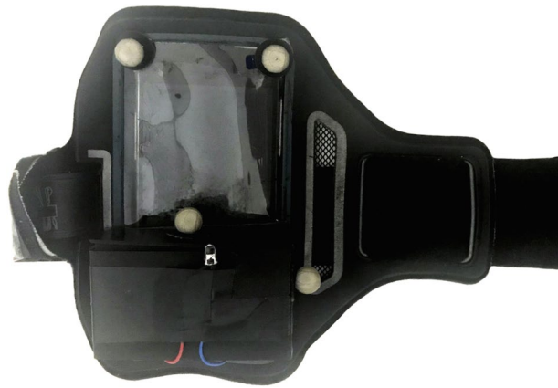
Fig. 2 The smartphone and MCU box mounted to a band to be attached to the leg.
