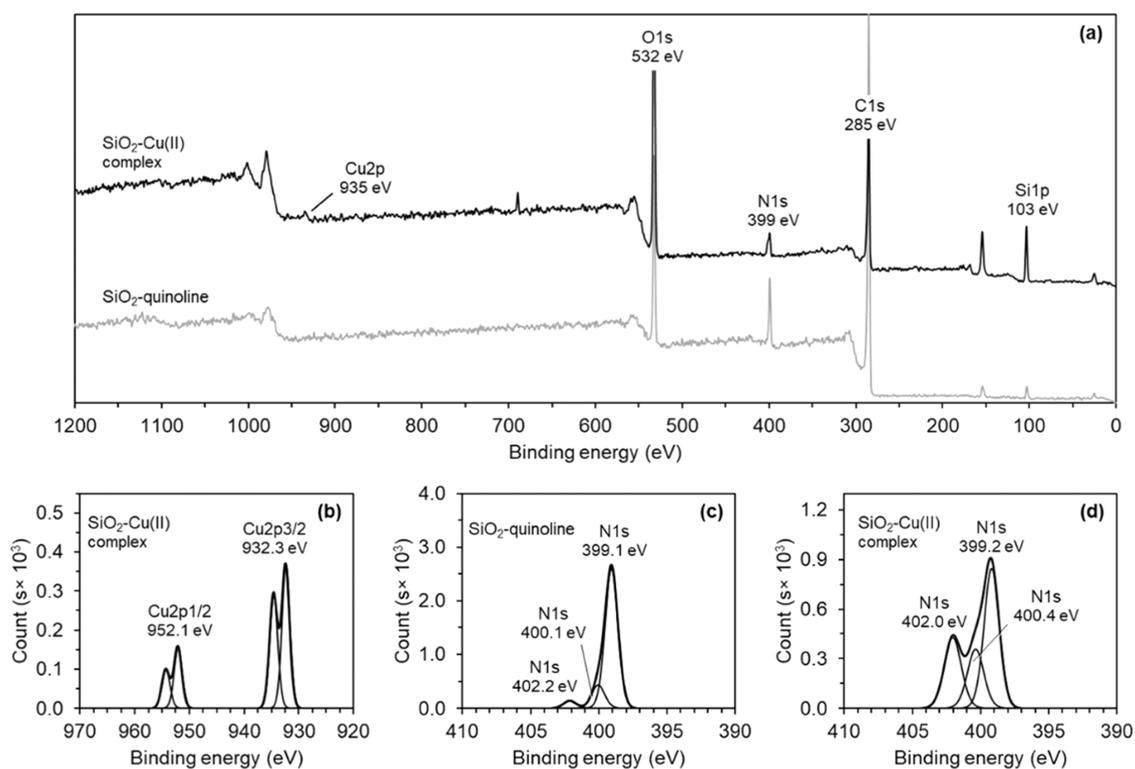
**Figure 5.** (a) XPS survey spectra of SiO<sub>2</sub>-quinoline before and after loading of Cu(II), and the high-resolution XPS for (b) Cu 2p and N 1s (c) before and (d) after loading of Cu(II).
