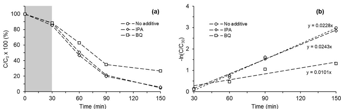
**Figure 11.** (a) Catalytic efficiency and (b) pseudo-first-order kinetic plot of the catalyst in the presence of radical active species-trapping agents.
