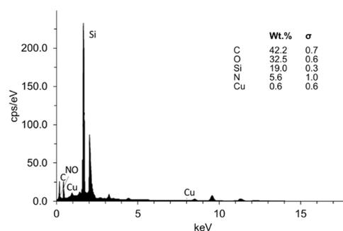
Figure 3. EDX spectra of the SiO<sub>2</sub>-Cu(II)-quinoline complex.
