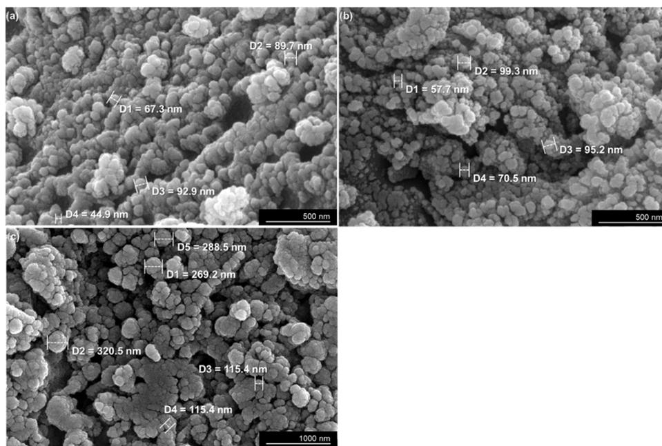
Figure 1. SEM images of (a) SiO<sub>2</sub>, (b) SiO<sub>2</sub>-NH<sub>2</sub>, and (c) SiO<sub>2</sub>-Cu(II)-quinoline complexes.
