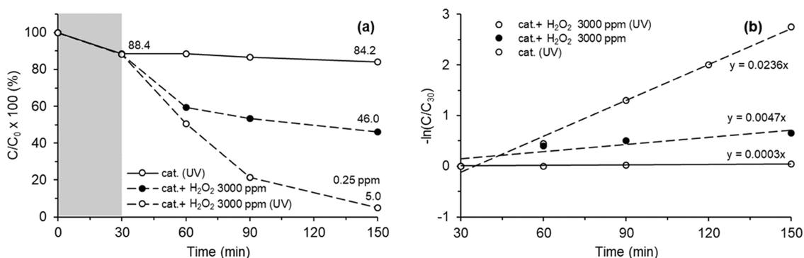
**Figure 7.** (a) Catalytic efficiency and (b) pseudo-first-order kinetic plot for the degradation of MB in different reaction systems.
