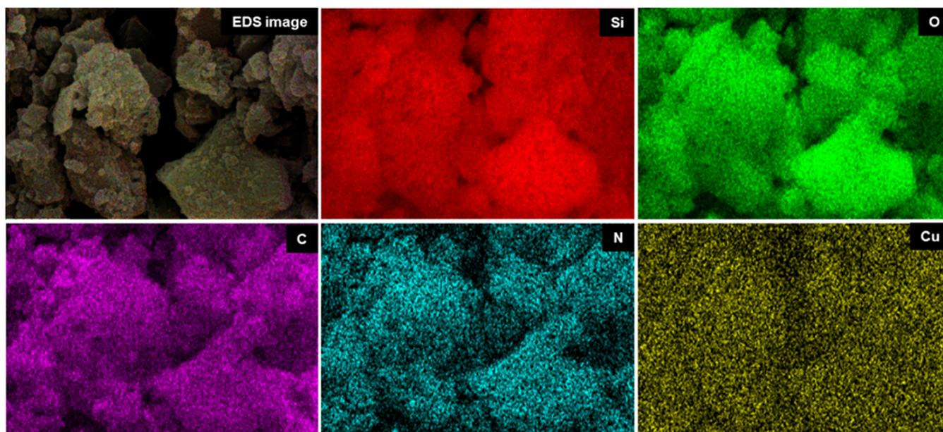
Figure 2. EDX mapping of the SiO<sub>2</sub>-Cu(II)-quinoline complex.
