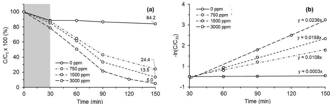
Figure 9. (a) Catalytic efficiency and (b) pseudo-first-order kinetic plot for degradation of MB using different concentrations of  $\text{H}_2\text{O}_2$ .
