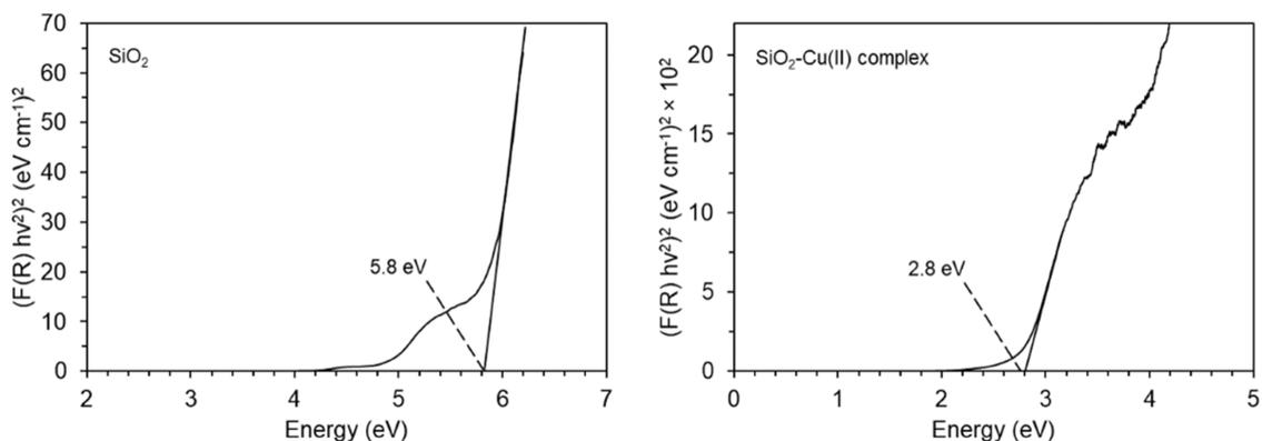
**Figure 6.** Kubelka-Munk function of (a) SiO<sub>2</sub> and (b) SiO<sub>2</sub>-Cu(II)-quinoline complexes.
