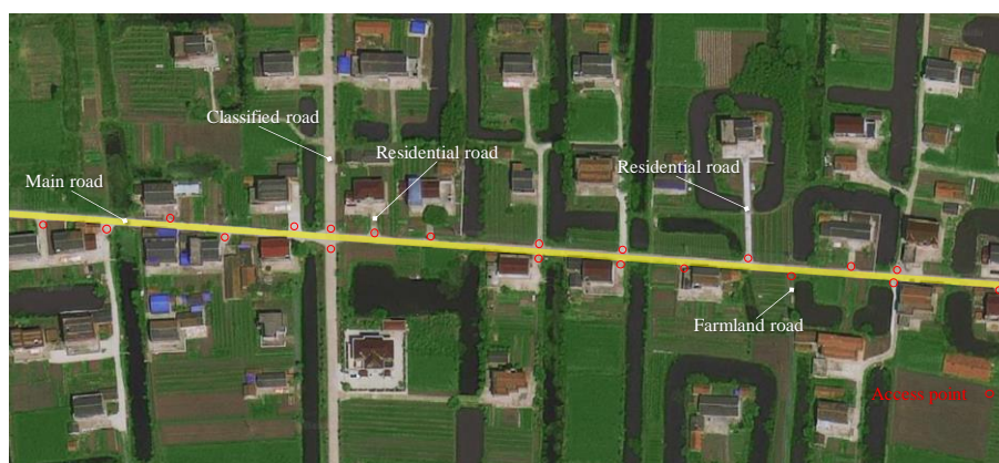
Figure 2. Definition of access point.
