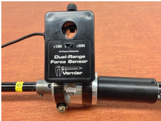
Figure 9 The force sensor attached to the extension knob of the DTEM.
