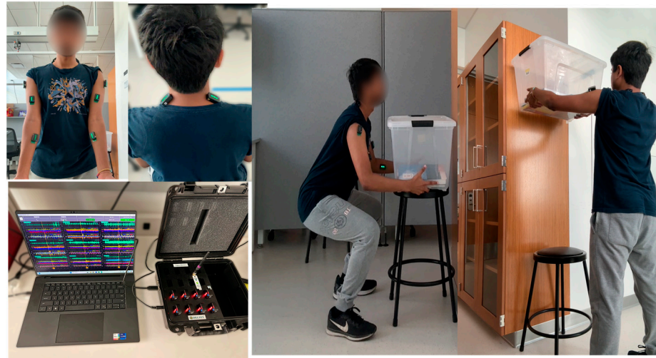
Figure 3. Data collection and experimental setup using DelSys sensor system.
