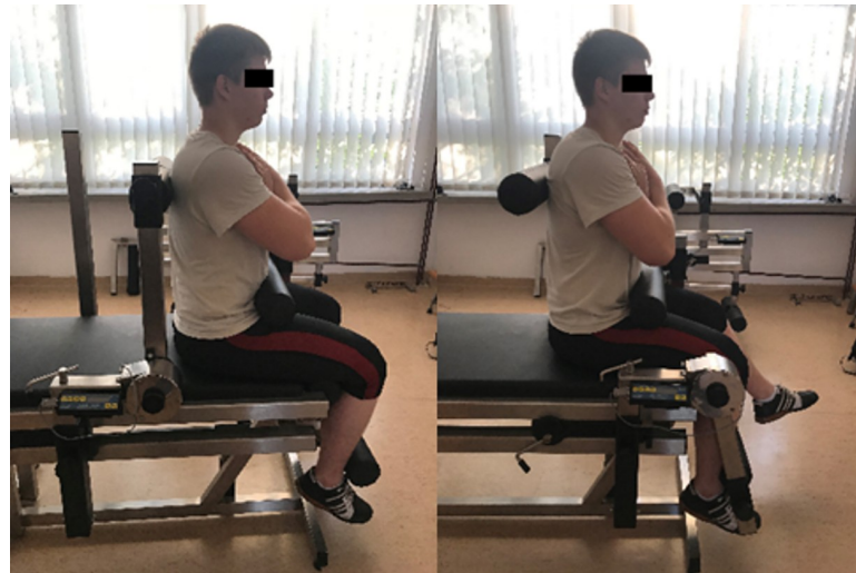
Fig 2. Measurement of peak torque of trunk extensors (left) and knee extensors (right) in isometric conditions.
