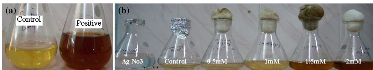
Fig. 1 a Showing the formation of silver nanoparticles after 48 h of incubation. b Effect of various concentrations of silver nitrate AgNO 3 on nanoparticle synthesis
