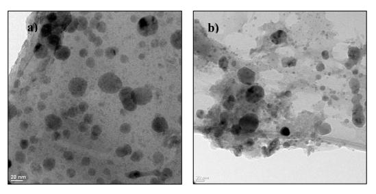
Figure 2. TEM micrography of selenium (a) and copper (b) nanoparticles.
