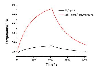
**Figure 7.** Temperature profile recorded on a suspension of PMLABe NPs incorporating 10 wt% of Ni8C12 complexes in water ( $C_{pol} = 300 \ \mu g \cdot mL^{-1}$ ) under 880 nm laser irradiation (17 min irradiation 3 W·cm<sup>2</sup> + 17 min laser OFF).
