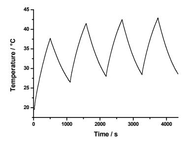
**Figure 9.** Stability measurement on a suspension of PMLABe NPs incorporating 10 wt% of Ni8C12 complex ( $C_{pol} = 300 \ \mu g \cdot m L^{-1}$ ) over three heating cycles under 880 nm laser irradiation (3 W·cm<sup>-2</sup>).
