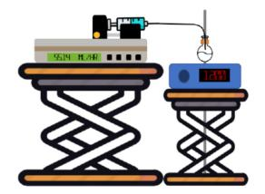
**Scheme 2.** Drawing of the setup used, constructed from a Fisherbrand<sup>™</sup> KDS100 Legacy syringe pump and 2 mL plastic syringes with Sterican (0.80 mm × 120 mm) hypodermic needles for injection into a 10 mL glass round-bottom flask placed over a Heidolph MR Hei-Tec magnetic stirrer.
