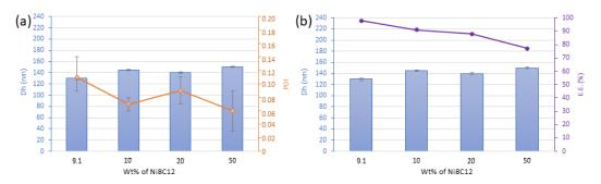
**Figure 5.** (a) Evolution of NPs hydrodynamic diameter (Dh) and dispersity (PDI) measured by DLS, as a function weight percent of Ni8C12, and (b) evolution of NP hydrodynamic diameter (Dh) and encapsulation efficiency (E.E.) as a function weight percent of Ni8C12 (for E.E., only one measurement was performed).
