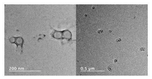
**Figure 3.** TEM images of the PMLABe<sub>73</sub> NPs obtained at a stirring rate of 1200 rpm, a polymer concentration of 5 mg/mL, an addition rate of 55.14 mL/h and a THF:water ratio of 1:2.
