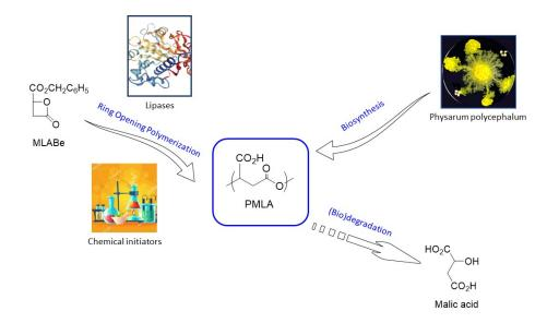
Figure 1. Structure of PMLA, methods of (bio)synthesis and degradation product.
