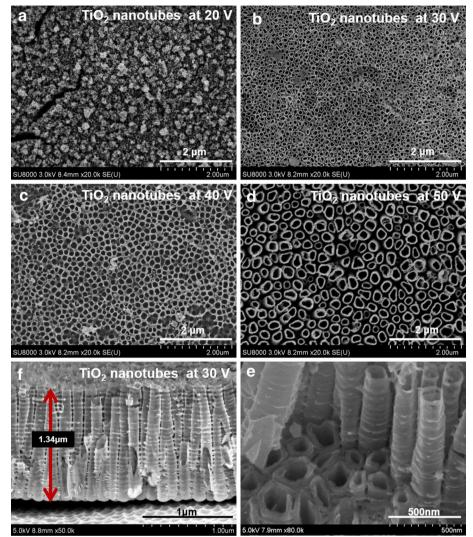
**Fig. 1** Representative surface morphology images of  $TiO_2$  nanotubes under different voltage: **a** 20 V, **b** 30 V, **c** 40 V and **d** 50 V. The diameters of the nanotubes fabricated under 30 V, 40 V and 50 V were, respectively (98.4 $\pm$ 11.4) nm, (136 $\pm$ 21.9) nm and (238 $\pm$ 33.5) nm, respectively. **e**, **f** Cross-sectional view of mechanically fractured sample showing that the length of the tubes was approximately 1.34 $\pm$ 0.26  $\mu$ m
