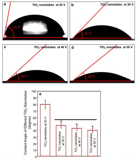
**Fig. 2** The wettability of  $TiO_2$  nanotubes prepared under different voltage. Contact angles as measured on a  $TiO_2$  nanotubes at 20 V, **b**  $TiO_2$  nanotubes at 30 V, **c**  $TiO_2$  nanotubes at 40 V, **d**  $TiO_2$  nanotubes at 50 V. **e** The contact angles for each group (mean  $\pm$  SD, n = 6). Bars with dissimilar letters indicate significantly different values (p < 0.05)
