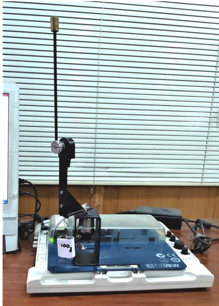
Fig 11. The QNET Rotary Pendulum's hardware setup.
