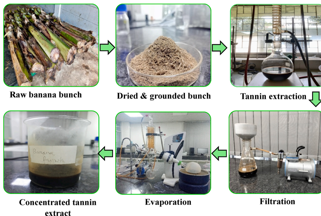
Fig. 1. Schematic extraction diagram of banana bunch tannin.
