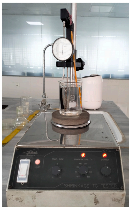
Fig. 10. Shrinkage temperature testing.
