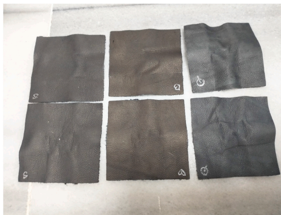
Fig. 9. Wrinkles development after flexing endurance testing of bunch extract (B), syrup (S), and quebracho (Q) tanned leather.
