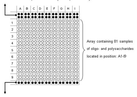
One row of ink printed to identify the bottom of the array
