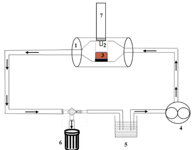
**Fig. 2.** Schematic view of the setup of one complete specimen chamber in an ex-vivo bioreactor system 1. Specimen chamber, 2. Polycarbonate holder, 3. Bone Core, 4. Peristaltic pump, 5. Media container, 6. Waste container, 7. Pneumatic Actuator.
