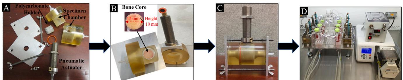
**Fig. 1.** Ex-Vivo Bone Bioreactor System. A) Individual components of a Specimen chamber, including specimen chamber, polycarbonate holder, pneumatic actuator, holders and wing nuts. B) Loading mechanism for a bone core (Diameter 15 mm and Height: 10 mm) into the specimen chamber C) Assembled Specimen Chamber. D) Complete assembly of an ex-vivo bone bioreactor system with 8 specimen chambers with a peristaltic flow pump, media containers and waste container.
