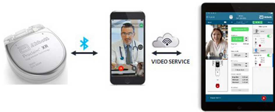
Figure 1 System used for remote care. Implanted neuromodulation device connects wirelessly to the iPhone patient controller using Bluetooth. The patient controller establishes an internet connection to the iPad clinician programmer with integrated audio and video. The clinician programmer has an inset video of the patient and access to the full set of programming controls.
