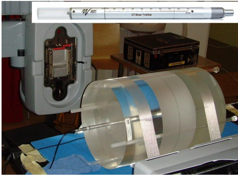
FIG. 4. CT Dose Profiler in the measurement setup. Three CTDI body phantoms joined together, with a CT Dose Profiler detector placed in the central hole. Upper right: the CT Dose Profiler.
