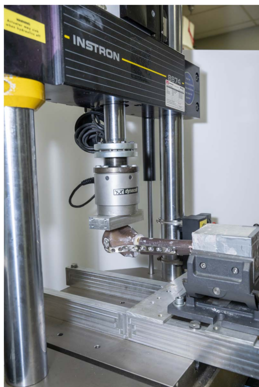
Fig. 3 A lateral tibial plateau plate with locking screws has been applied to a synthetic proximal tibial fracture model. An external fixator hole has been drilled distal to the most distal locking screw in the plate. The Instron unit applied force directed from posterior to anterior on the proximal tibia.
