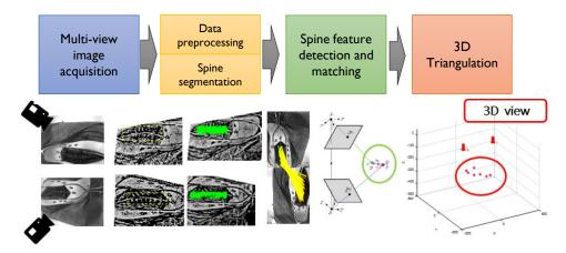
Figure 3. Proposed framework for 3D spine feature localization.
