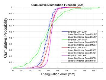
**Figure 12.** Cumulative distribution function (CDF) of the triangulation error for the four methods. The dotted area delimits the 95% confidence interval for each CDF. The triangulation error of the analyzed frames is lower than 0.5 mm in more than 97% (SURF) or 95% (FAST and ORB). For MSER, however, the corresponding number is 84%, likely explained by the larger variability in triangulation errors.
