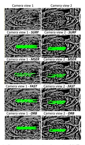
**Figure 8.** Detection of spine features in two image views (camera 1 and 2). The numbered views above the two columns of images, refer to the two cameras. In the first row the preprocessed images are shown. The subsequent rows illustrate results after applying the four feature detection algorithms (SURF, MSER, FAST and ORB). Green is used to indicate salient spine features identified by the respective algorithms.
