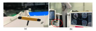
**Figure 1.** Images of standard setup with indirect patient tracking ([18]). (a) The stereoscopic infrared camera setup for tracking the DRF (dynamic reference frame). (b) The DRF (in the red circle) and the monitor displaying the position on a CT patient scan.
