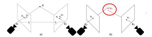
**Figure 6.** (a) An ideal triangulation where  $C_1$  and  $C_2$  define the 3D positions of Cameras 1 and 2, respectively. The 3D Triangulation of point X is projected into two camera views in the points  $x_1$  and  $x_2$ , (b)  $V_p$  is the line segment representing the shortest distance between to two back-projected lines.
