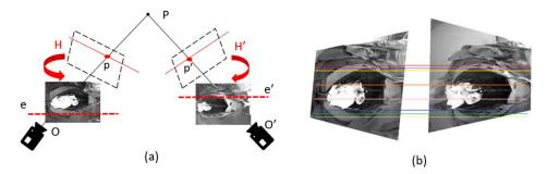
**Figure 4.** Image rectification, (a) the projective transformation *H* lead the matching of the epipolar lines. (b) shows an epipolar geometry matching after image rectification, the epipolar lines plotted for the optical markers run parallel after image rectification.
