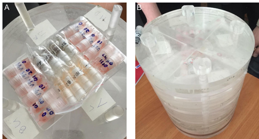
Fig. 1. The samples in 2 ml vials (A) placed in the plexiglass phantom (B).
