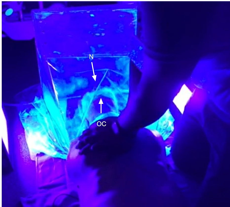
FIGURE 5: Performing chest compressions with our nebulized mannequin model under blacklight
