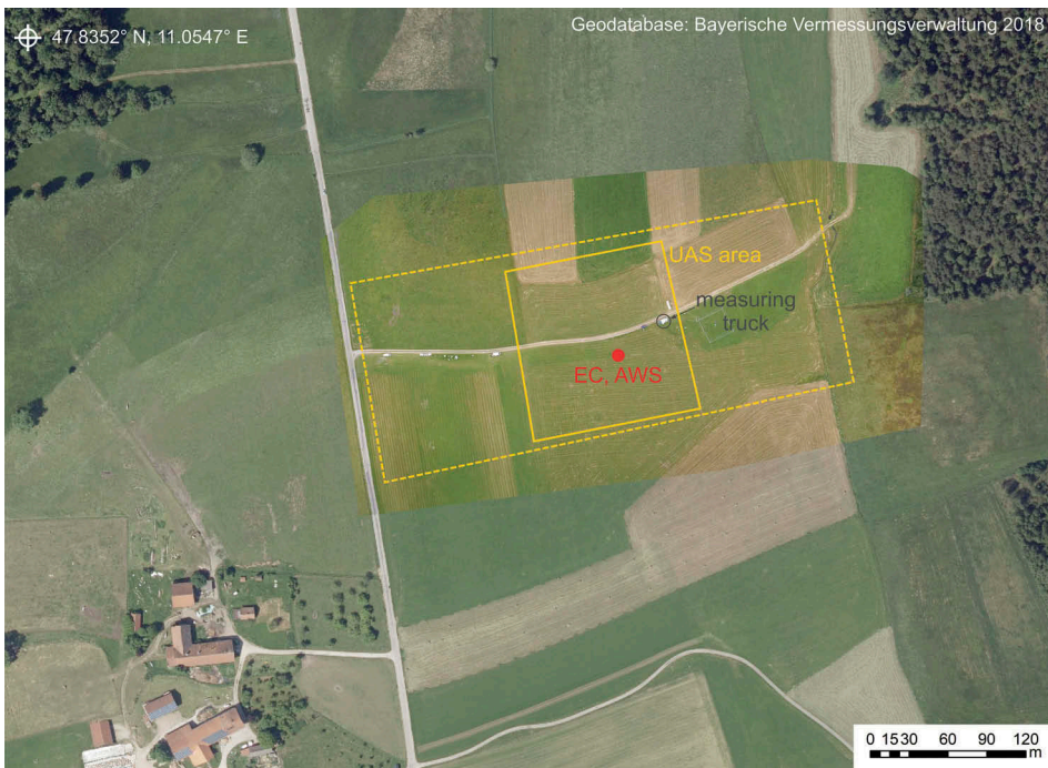
Figure 1. Overview of the study area using an orthophoto (© Bayerische Vermessungsverwaltung – the Bavarian Agency for Surveying and Geoinformation) superimposed by an UAS-based RGB image acquired on 11 July at a flying altitude of 100 m. The red marker indicates the location of the EC tower. The solid yellow line sketches the area covered by the thermal imager for the flights at an altitude of 25 m. The dashed yellow line corresponds to the area covered with the flights at 100 m altitude. The exact extent of the thermal orthomosaic varied from flight to flight.
