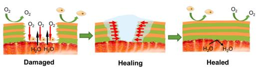
Figure 4. Diagram of self-healing behavior of chitosan (CS)/sodium alginate (SA) coating.
