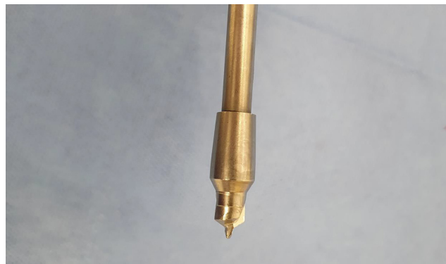
Figure 4 Example of the drill utilized for acetabulum cement hole creation.
