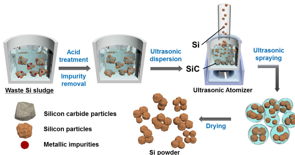
Figure 1 | Schematic drawings illustrating the ultrasonic aerosol assisted Si extraction process.
