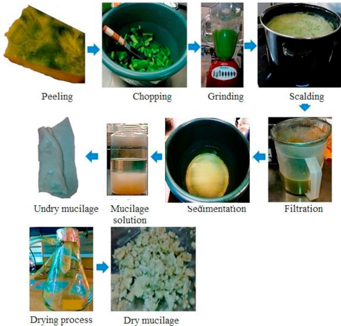
Figure 2. Stages of the extraction process of Opuntia ficus mucilage.
