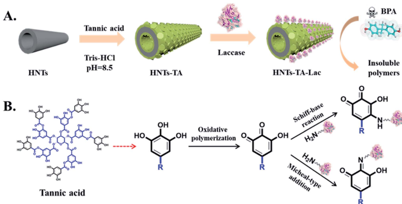
Scheme 1 Schematic of (A) fabrication process of HNT-TA-Lac for the removal of BPA and (B) the mechanism of laccase immobilization.
