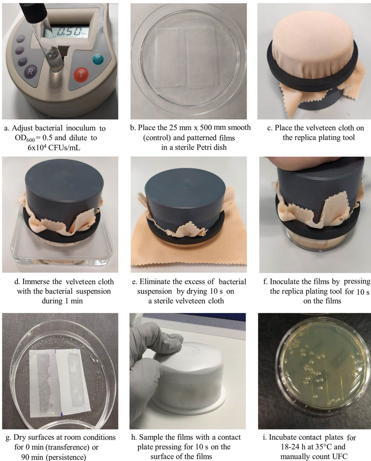
Figure 3. Schematic representation of the touch-transfer assay.
