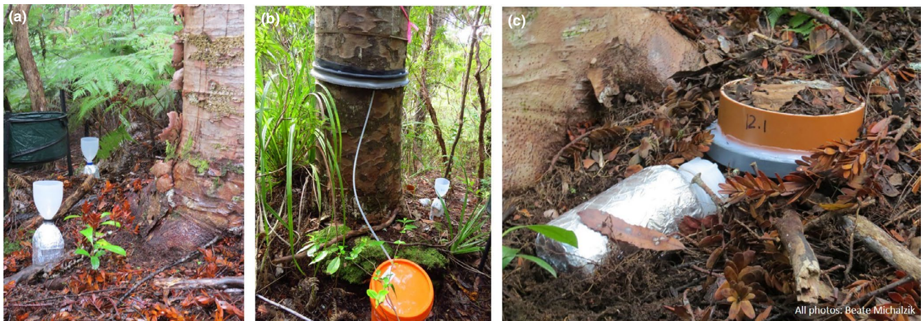
FIGURE 2 Canopy and forest floor leachate collectors: (a) throughfall, (b) stemflow, and (c) free-draining lysimeter
