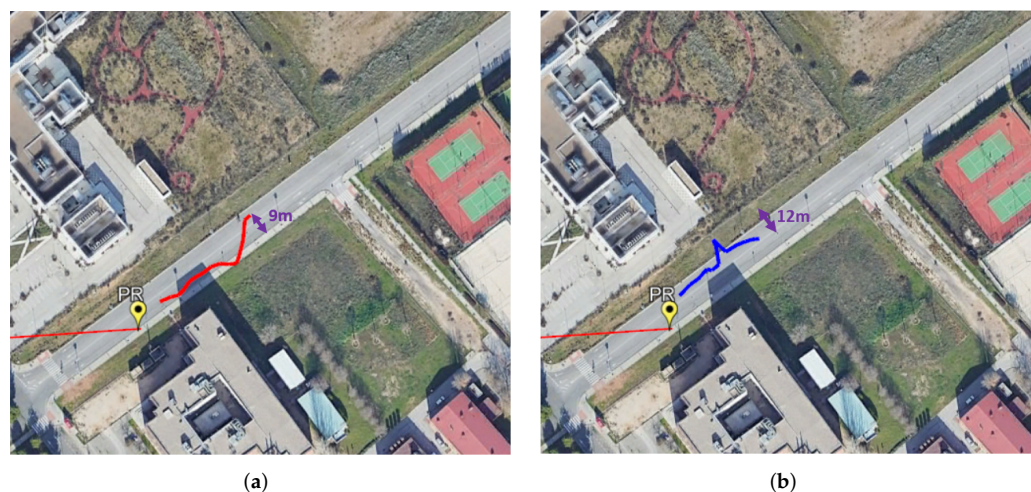
Figure 14. Localization results for non-cooperative targets moving away from PR location (blue and red). (a) First non-cooperative target. (b) Second non-cooperative target.
