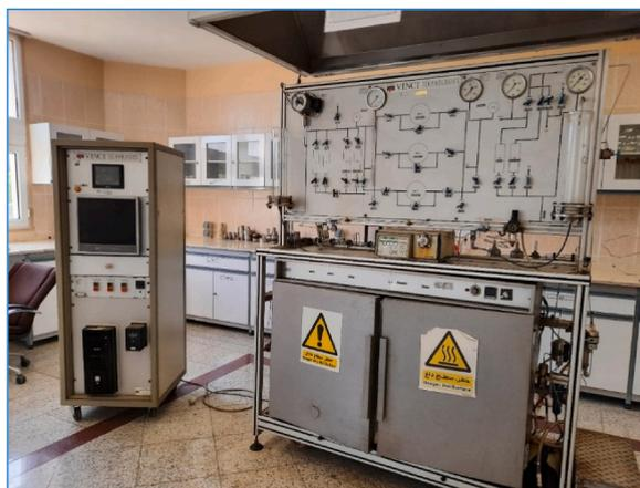
Fig. 4. Photograph of flooding assembly used in this work.
