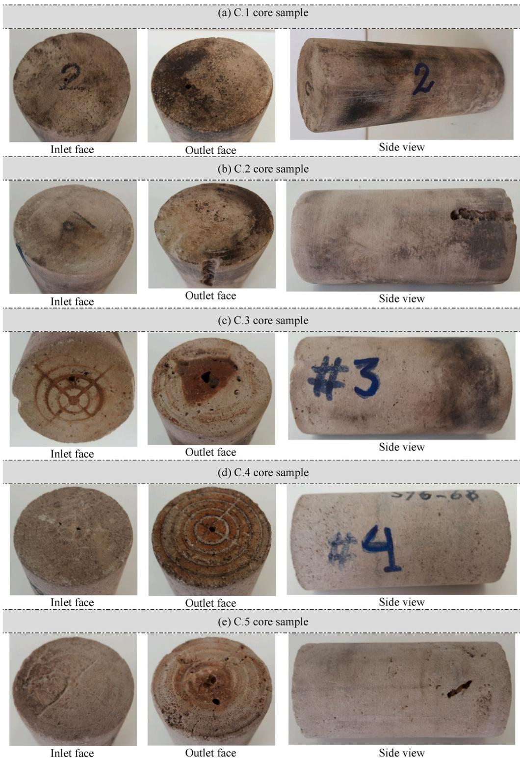
Fig. 10. Inlet, outlet, and side views of tested cores after acidizing: (a) C.1, (b) C.2, (3) C.3, (d) C.4, (e) C.5.
