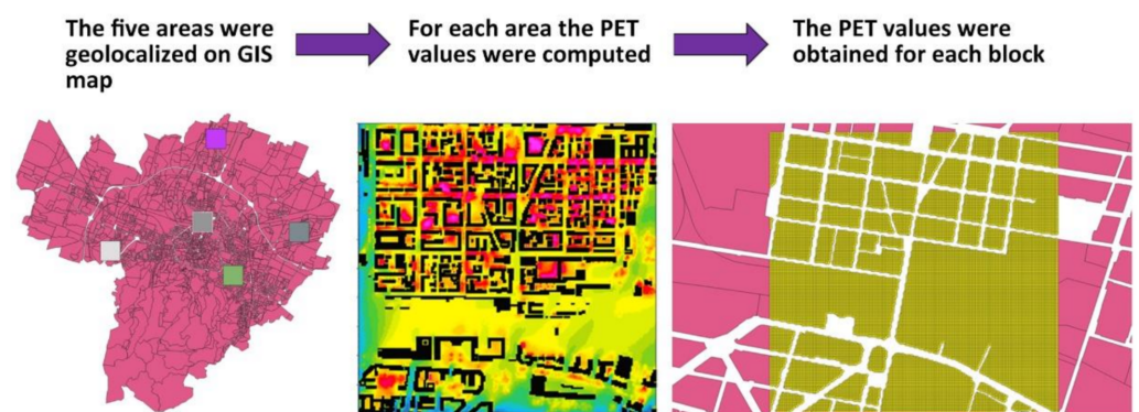
Figure 9. Geo-localization on GIS map of the five simulated areas, extraction of PET values from the model runs and computation of PET values for each “block”.
