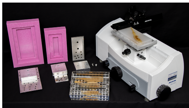
FIGURE 1 Equipment used for this technique. From left to right: Custom made silicon molds and mounting stages composed of a plate and a base, Pathcentre trays with tissues, sliding microtome. Aluminum mounting plates were made in two sizes to accommodate the varying tissue lengths, a 10 × 20 cm plate for larger specimens and a 6.5 × 15 cm plate for smaller specimens. The processor, Leica ASP300S Pathcentre, is not shown in this image
