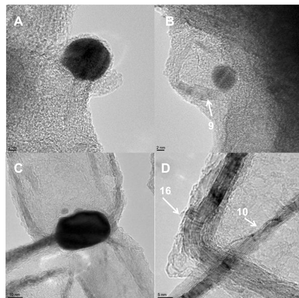
Figure 2 High-resolution transmission electron microscopy (HRTEM) images of (A and B) the graphene-gold (1.0 wt%)-silver (1.0 wt%) (Gr-AuAg-1) composite and (C) graphene-gold (1.5 wt%)-silver 1.5 wt% (Gr-AuAg-1.5) composite showing metal nanoparticles located at the edge of the graphene sheet; (D) HRTEM image of the Gr-AuAg-1.5 composite showing the number of layers within graphene sheets.
