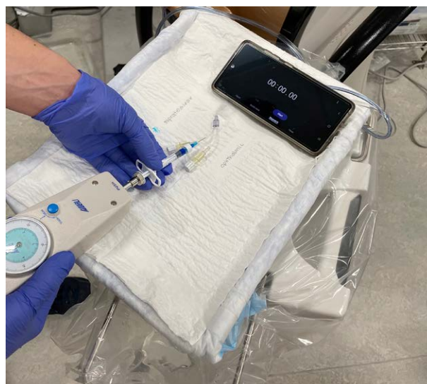
Fig. 1. Experimental setup design. The bifurcation tubing marked supratrochlear was punctured through the rubber stopper on the end of the leg with a 27G needle, whereas the rubber stopper on the leg marked ophthalmic was punctured with a 16G needle to simulate the difference in arterial sizes between the anatomic arteries. A dynamometer was used to keep the injection pressure constant at 22 Newtons. The filler was injected with a 27G and 30G needle through the tubing marked supratrochlear artery, and videography and stopwatch were used to measure the time for filler to cause antegrade flow and retrograde flow, and reach the bifurcation point.
