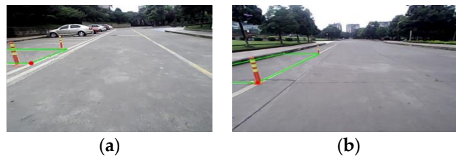
Figure 5. Matching of vertical and parallel parking spaces: (a) Matching on vertical parking space, (b) Matching on parallel parking space.
