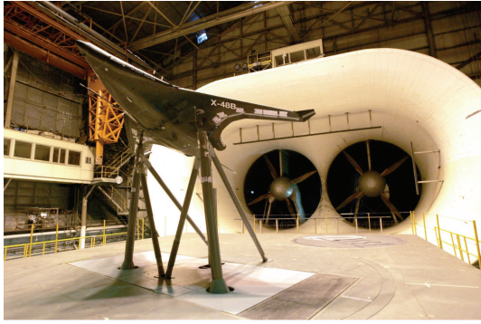
FIGURE 2: A common example of a prototype. A prototype of a blended wing body aircraft, the X-48B, is shown in a wind tunnel at NASA's research center in Langley Air Force Base, VA. The wind tunnel was used by researchers to evaluate this prototype against structural, aerodynamic, and operational design objectives for an advanced aircraft concept (NASA photo/Jeff Caplan).
