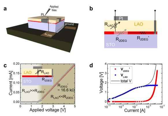
Figure 2 | (a) Schematic diagram of the Pt/LAO/STO capacitor devices. (b) A resistance equivalent circuit for the Pt/LAO/STO capacitor devices. (c) I–V curve of the device in a positive voltage region. The resistance of the device is considered to be the sum of the resistance of LAO layer and that of the 2DEG in the periphery of the capacitor. (d) Variation in the voltages applied to the LAO layer and the 2DEG in the vicinity of the capacitor.
