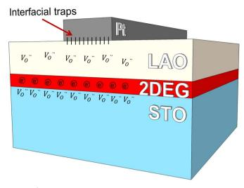
Figure 1  $\mid$  Schematic illustration of several kinds of defects in the Pt/ LAO/STO heterostructure.
