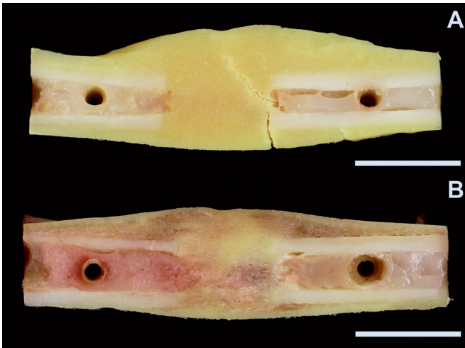
Figure 2. Longitudinal sections of the bone specimens made after the mechanical testing procedure: A. PTH; B. control. Bar = 10 mm.
