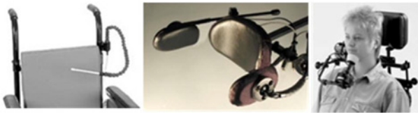
Fig. 1 Alternative types of powered chair control systems; sip and puff (left), head switch array (middle) and chin control (right) [2]
