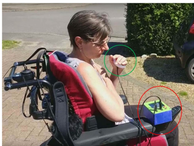
Fig. 10 Joystick manipulator (circled red) mounted on a powered wheelchair for final field testing, with the hand band mounted on the palm (circled green)
