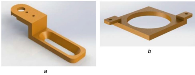
Fig. 4 The interface paddle and the main hole for the joystick control unit a Interface paddle – the primary mechanical contact between the joystick control unit and two-axis proportional joystick b Stem boss – centres the device over the powered chair joystick, ensuring accurate positioning
