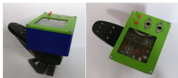
Fig. 3 Joystick control unit mounted on the test joystick jig
