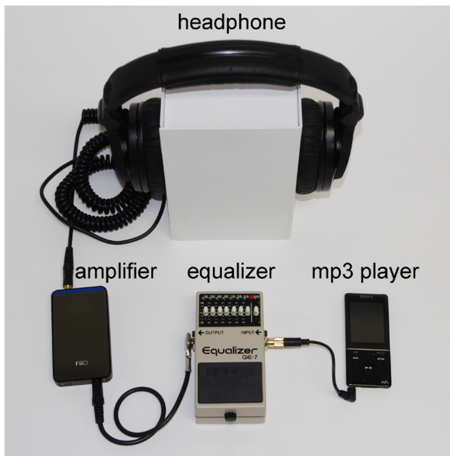
Figure 2. Connections and devices to use in CIST. A portable music player, equalizer, headphone amplifier, and closed-type headphone are sequentially connected. Equalizer and headphone amplifier are used only when the digital equalizer of the portable music player is not sufficiently effective. Please click here to view a larger version of this figure.
