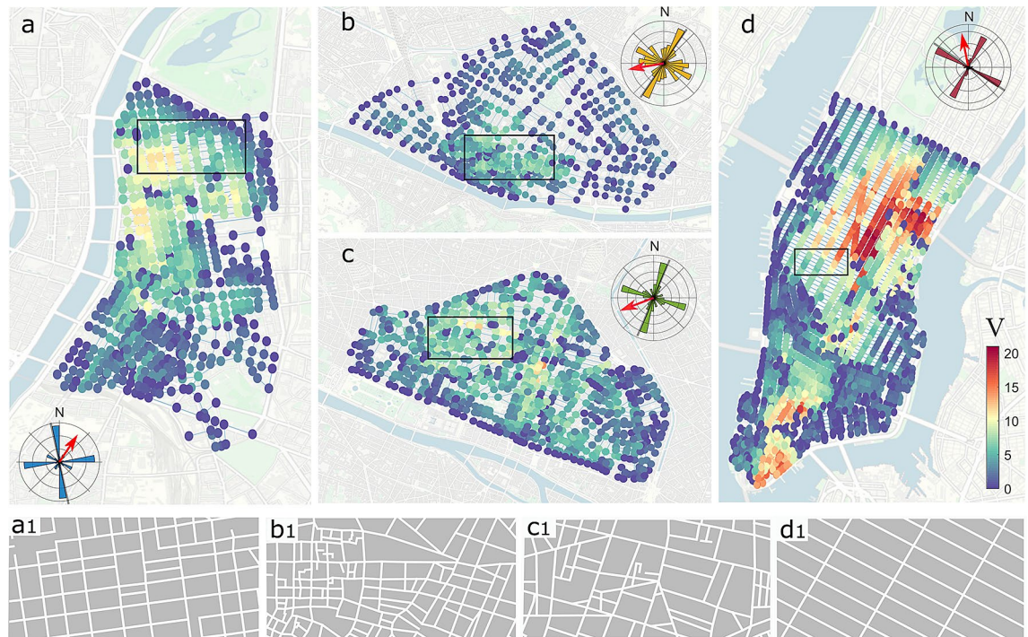
Figure 1. Vulnerability maps for (a) Lyon, (b) Firenze, (c) Paris, and (d) New York for a wind direction of 45^\circ with respect to the main axis of the urban fabric. The polar histograms in the insets report the distribution of street orientation, while the red arrows represent the wind direction with respect to the street network. Panels a1–d1 show the urban pattern in a rectangular area of 0.5 \text{ km}^2 (reported in panels a–d) for the cities of Lyon, Firenze, Paris, and New York, respectively. Background images made with QGIS 2.18 ( https://qgis.org ).
