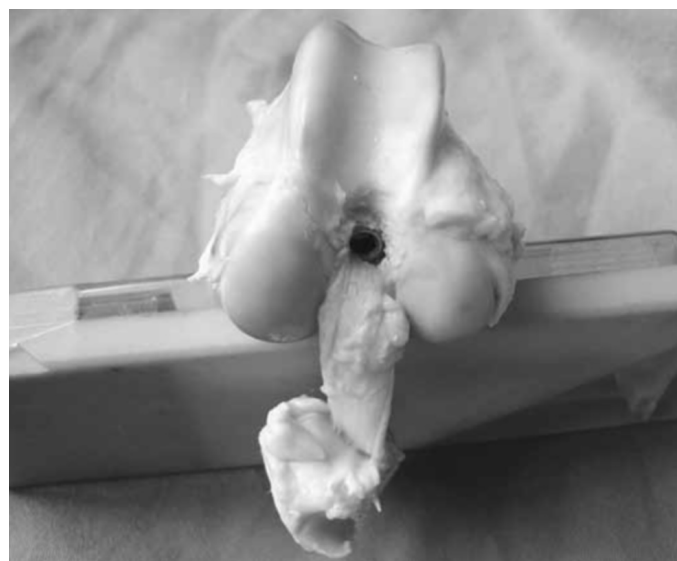
Figure 4 – Photograph of specimen fixed using interference screw.
